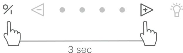
To switch the InTouch function off press the ① key and ② key at the same time for 3 seconds. The 2nd and 3rd LEDs flash 3 times to confirm. (The unit must be switched off).
