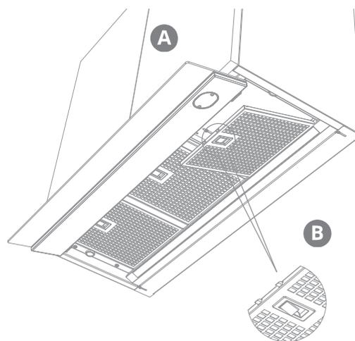
Open the rotating valve A. Protect the hob. You can take the grease filter B from the hood by pulling the handle on the filter. The filter will come down.
